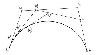
Graphically representing a cubic Bezier curve (degree 3) and the calculated point where t = 1/4.
