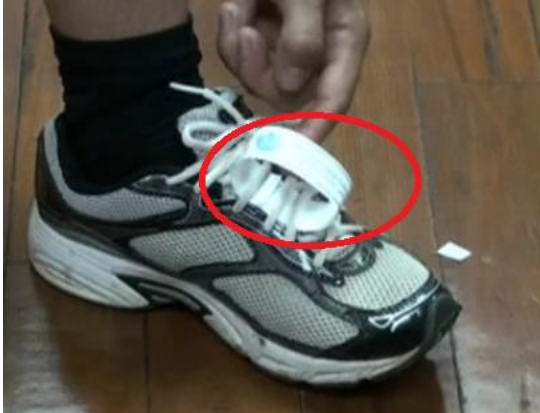
Fig. 2. UHF RFID tags attached to a shoe rope.
